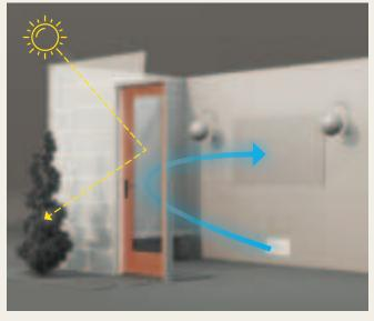
In warm weather, Low-E glass reflects the sun's rays off the glass and a home's air conditioning back inside to help keep the home cool.
